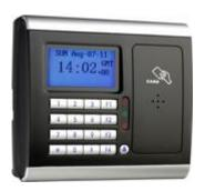
BF-831 is RFID identification based controller for proximity card. It is always used to manage entrance security, work place time attendance, overtime working verification and any other situation/ event for the authorized personnel's presence. It can either work standalone without connecting to the PC or be integrated with PC thru RS-232/485 or RJ-45 port. Also, BF-830 can be linked with BF-870 as a reader in Multi door control solution
